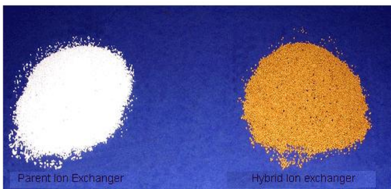
Figure 3 Parent Anion Exchange Resin (left) and hybrid anion exchanger (right) beads.
